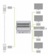
In this installation scenario, a single operator monitors several computers simultaneously, each with its own dynamically changeable display. Routing of the computers to the screens is achieved by means of a KVM matrix switch, such as the Draco tera enterprise or compact switch. Normal setup and operational procedures are used to configure the matrix of computers and screens separately.
