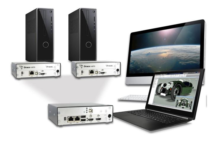
Accept KVM data from two remote transmitters while allowing access to a local computer at the receiver for full access to three sources using a single keyboard and mouse
