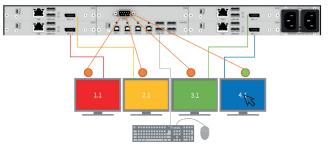
Multi-Screen Control with dry contact push button trigger to indicate active screen
