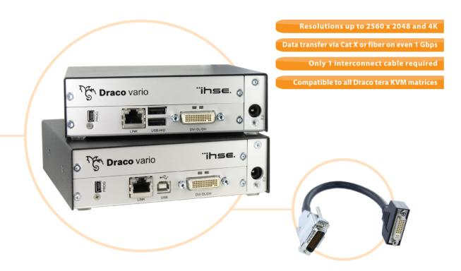
**THE DRACO VARIO DUAL LINK** enables the transmission of 4K video signals to one single monitor up to 4096 x 2160 and 3840 x 2160 at 30 Hz frame rate in addition to the usual 2560 x 2048 at 60 Hz and lower. Extension of signals requires a single Cat X or fiber cable link. Special monitor
